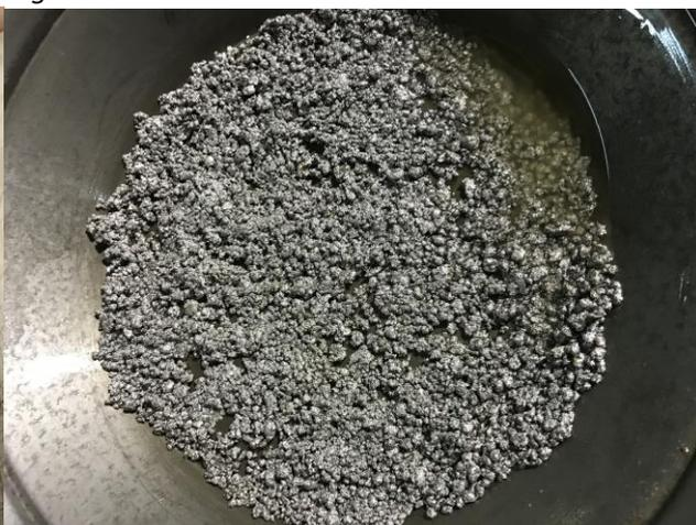
Figure3 on the left shows one of Thursday's batches of wet amalgam **weighing 1600g** and Figure4 on the right the same amalgam in the panning dish.
