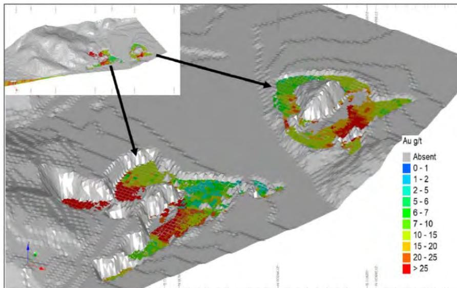
Figure 9) Modelled pit shells contained 335koz @ 16.9g/t Au (Source: Minxcon)
