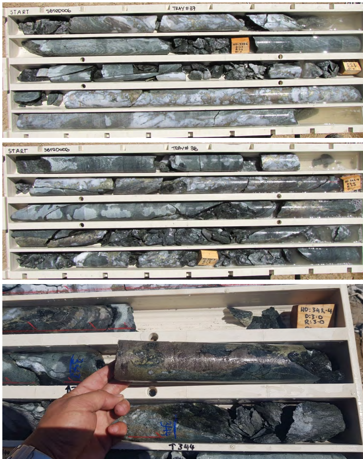
Figure 19. Bottletree SBTRD006 core: Top and middle photographs showing Trays 37 and 38 containing drill core from down hole depths 337m – 341.5m (approx.) and 341m – 344.5m (approx.) respectively, showing strong chalcopryite and pyrite mineralisation. Bottom photograph shows close-up view of drill core from 343m (approx.).
