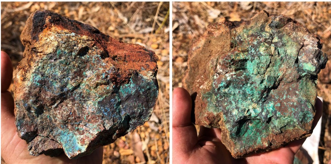
Figure 1: Rock chips CHWR01 (L) 25.6% Cu, 678g/t Ag and 1.3 g/t Au and CHWR02(R) 26.7% Cu, 371 g/t Ag and 0.5 g/t Au from the outcropping copper rich gossan at the Rufina North target located at ~610815E, 8167715N GDA94 MGAz51
