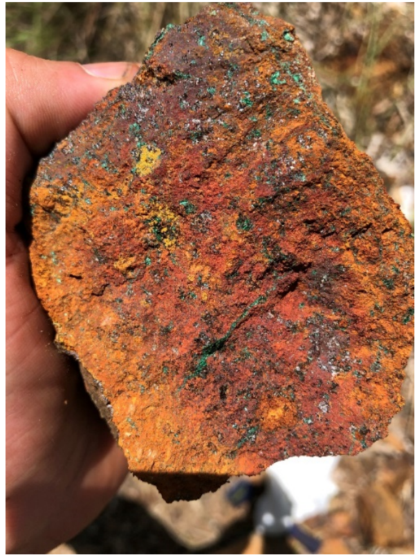
Figure 6: Sample CH25, malachite and copper oxide gossan. (GDA94 MGA 611889E, 8167112N) 16.1% Cu, 0.1% Pb, 0.3% Zn, 62g/t Ag, 0.4% Sn
