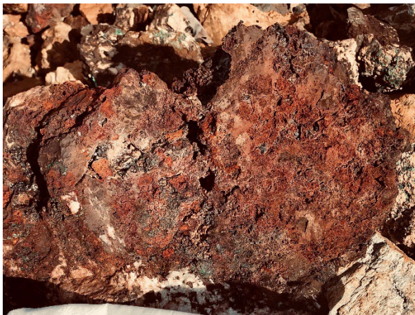
Figure 15: Sample GR19, Gossanous ironstone with trace malachite. (GDA94 MGA 628909E, 8168420N) 3.2% Cu, 1.2g/t Au, 1.0g/t Ag
