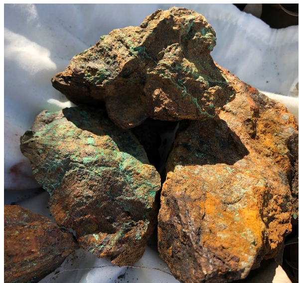
Figure 8: Sample CH07, malachite and jarosite stained gossan. (GDA94 MGA 628874E, 8168360N) 13.2% Cu, 0.1% Pb, 0.2% Zn, 13 g/t Ag, 0.3% Sn
