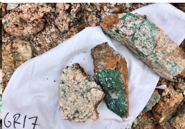
Figure 18: Sample GR17, Quartz and malachite vein. (GDA94 MGA 628909E, 8168420N) 4.2% Cu, 0.1g/t Au, 1.3g/t Ag
