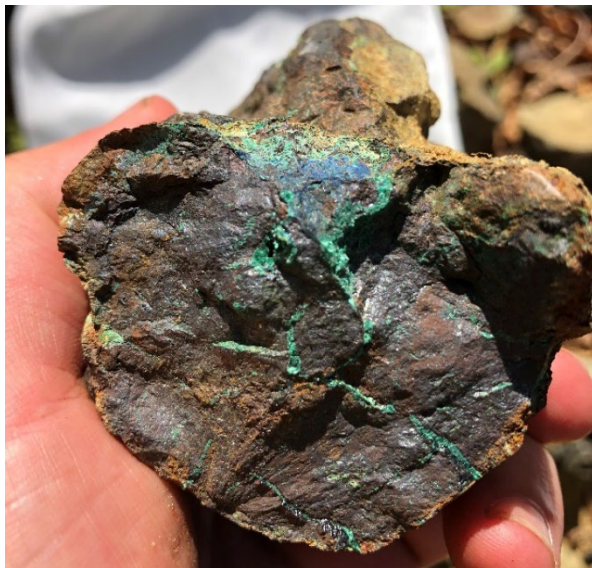
Figure 7: Sample CH02, azurite and malachite stained gossan. (GDA94 MGA 611871E, 8167056N) 10.4% Cu, 0.1% Pb, 0.2% Zn, 29 g/t Ag 0.1% Sn
