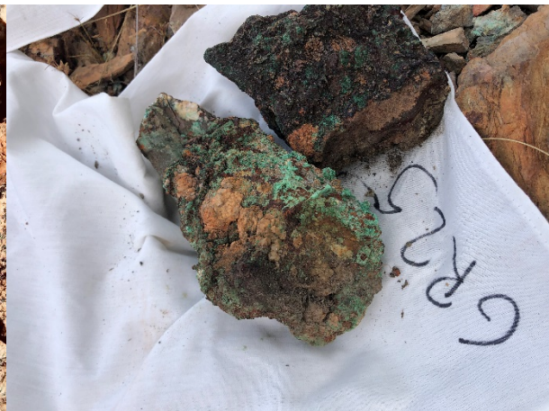
Figure 16: Sample GR25, Quartz with malachite and copper oxides. (GDA94 MGA 628874E, 8168360N) 27.3% Cu, 0.6g/t Au, 1.6g/t Ag
