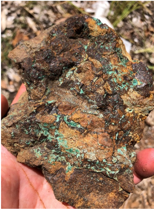
Figure 5: Sample CH23, malachite stained gossan. (GDA94 MGA 611890E, 8167099N) 19.2% Cu, 0.1% Pb, 0.1% Zn, 37g/t Ag
