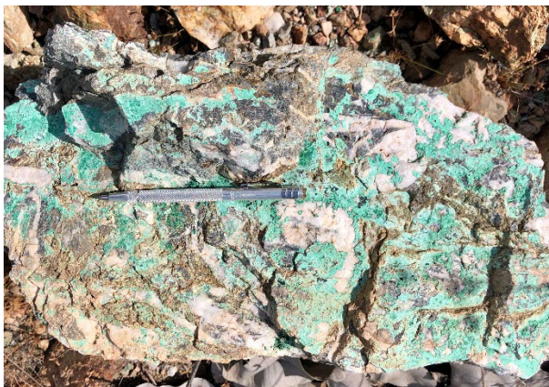
Figure 17: Sample GR20, Silicified slate with quartz veining and malachite. (GDA94 MGA 628903E, 8168397N) 12.4% Cu, 0.2g/t Au, 1.7g/t Ag
