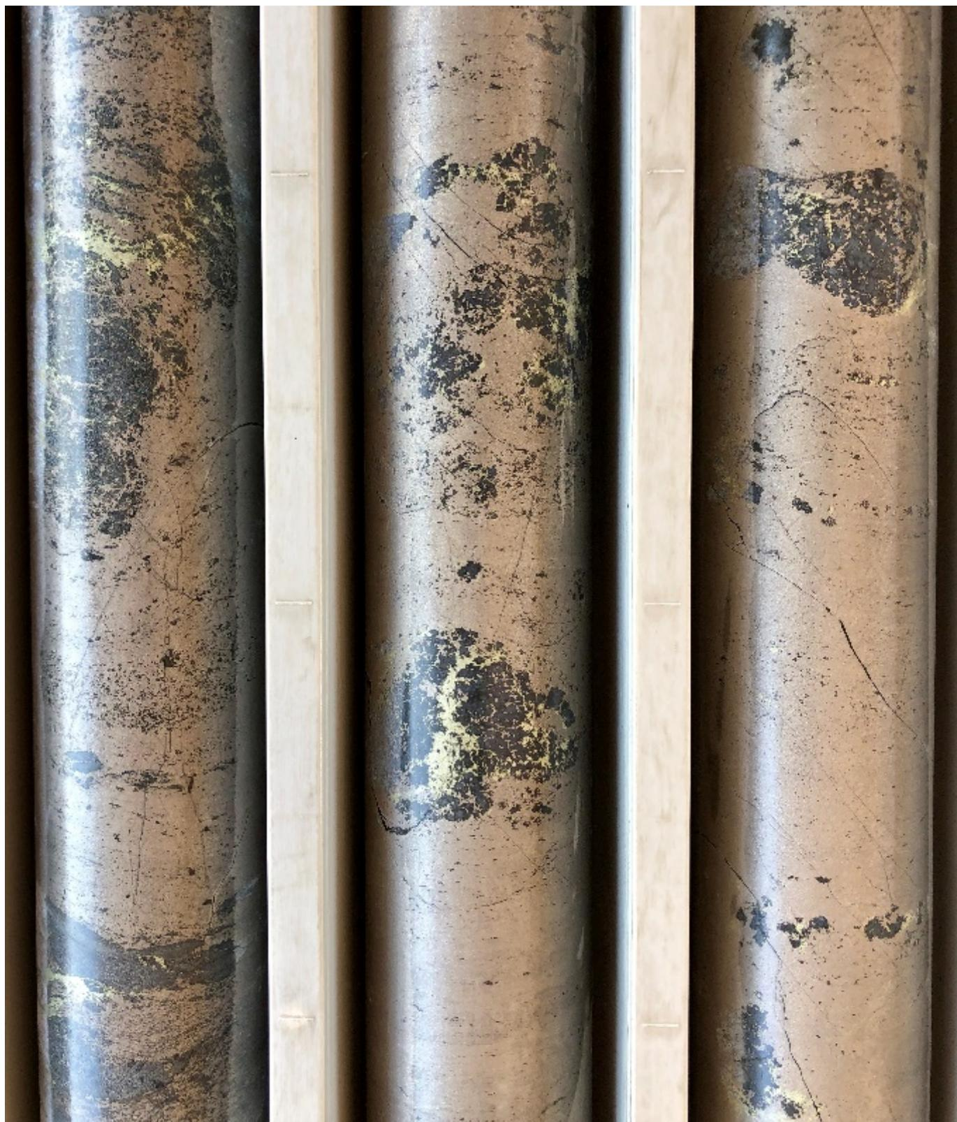
***Figure 4: Massive sulphides from the lower zone (po, cp)***
