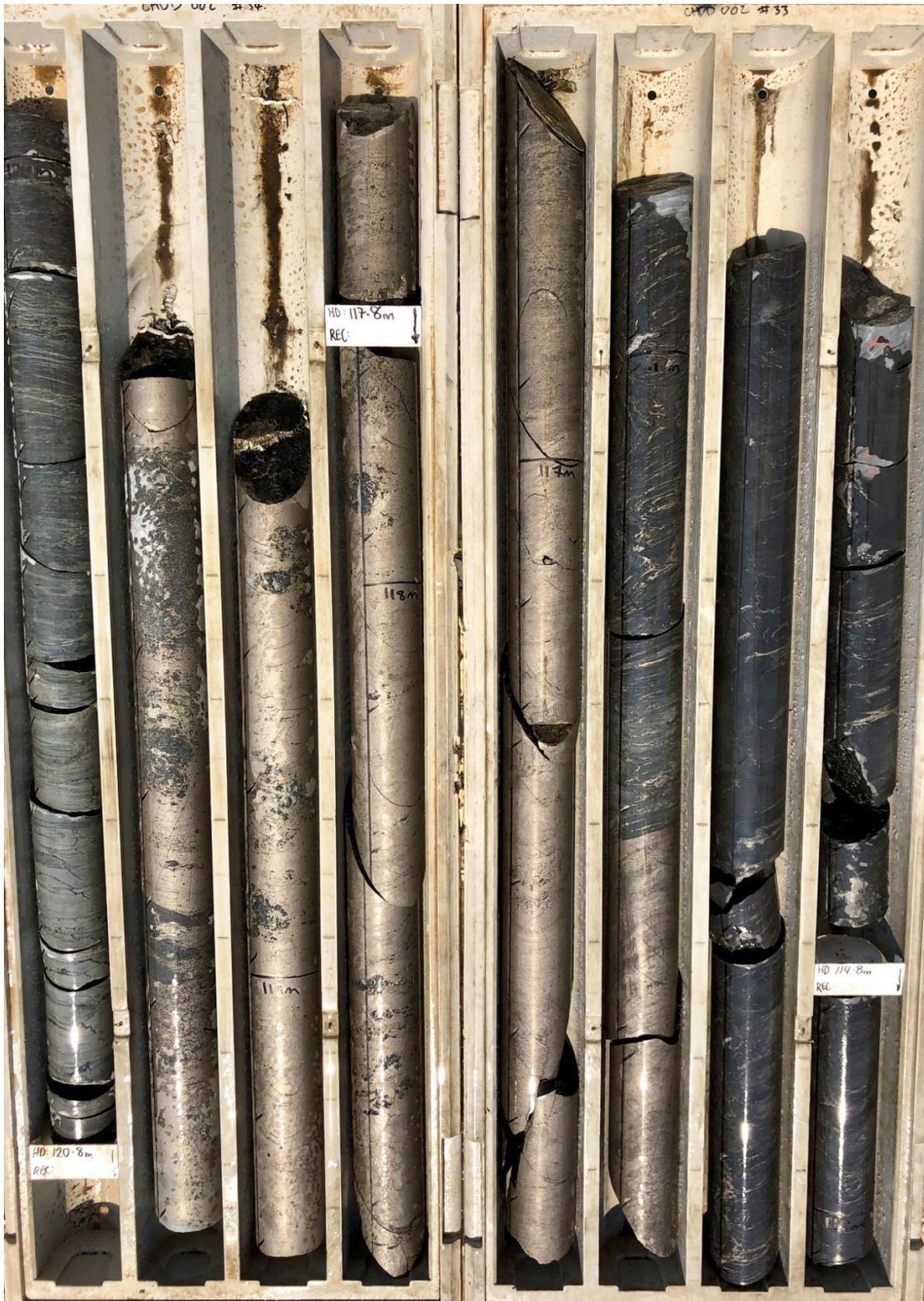
**Figure 6: Massive sulphides in the Lower Zone (po, cp, sp)**
