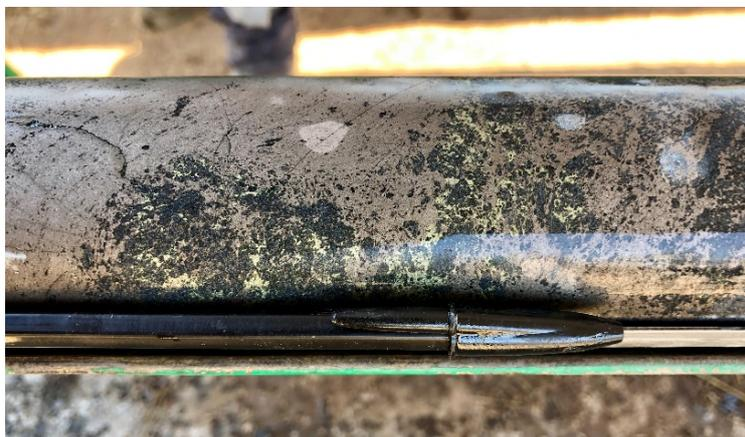
**Figure 1: Massive sulphide showing chalcopyrite and pyrrhotite.**
