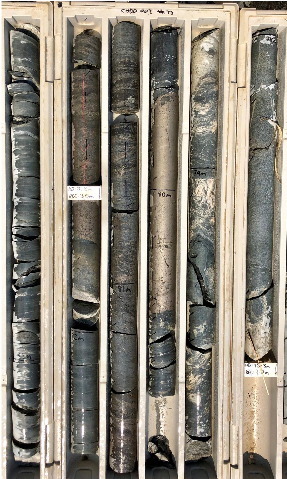
**Figure 5: Massive and semi massive sulphides from the Upper Zone (po, cp, sp).**
