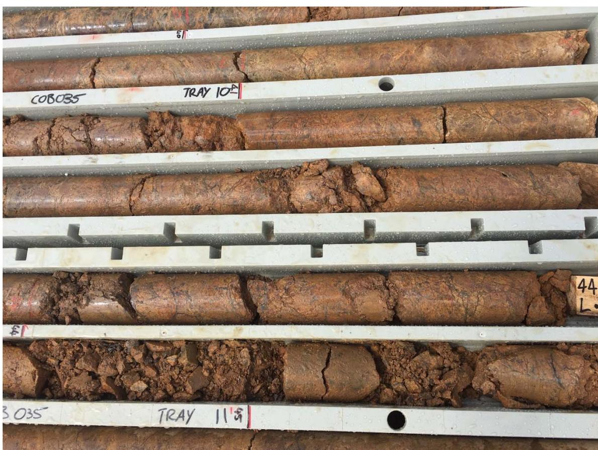
Figure 2 – Drill core (COB035) highlighting shear zone (fractured zones)
