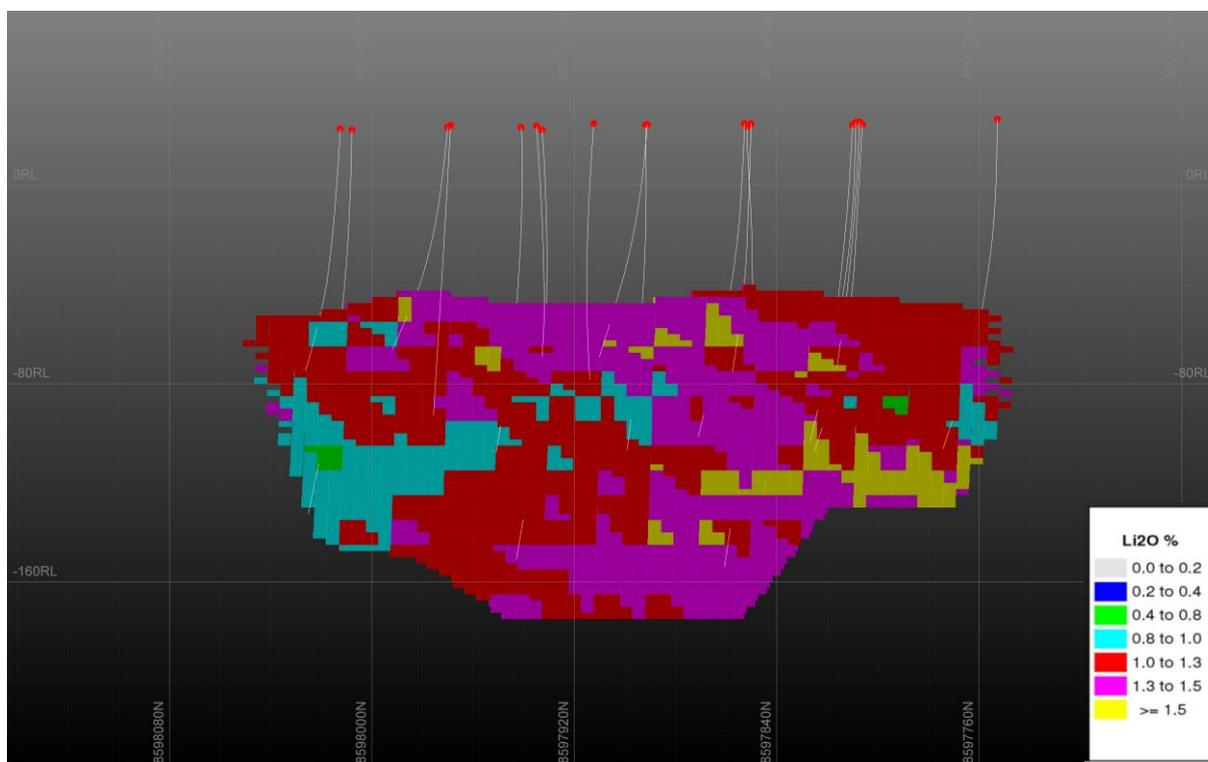
**Figure 2.** Lithium Grade (% Li<sub>2</sub>O) block model for Carlton Mineral Resource, Finnis Lithium Project.
