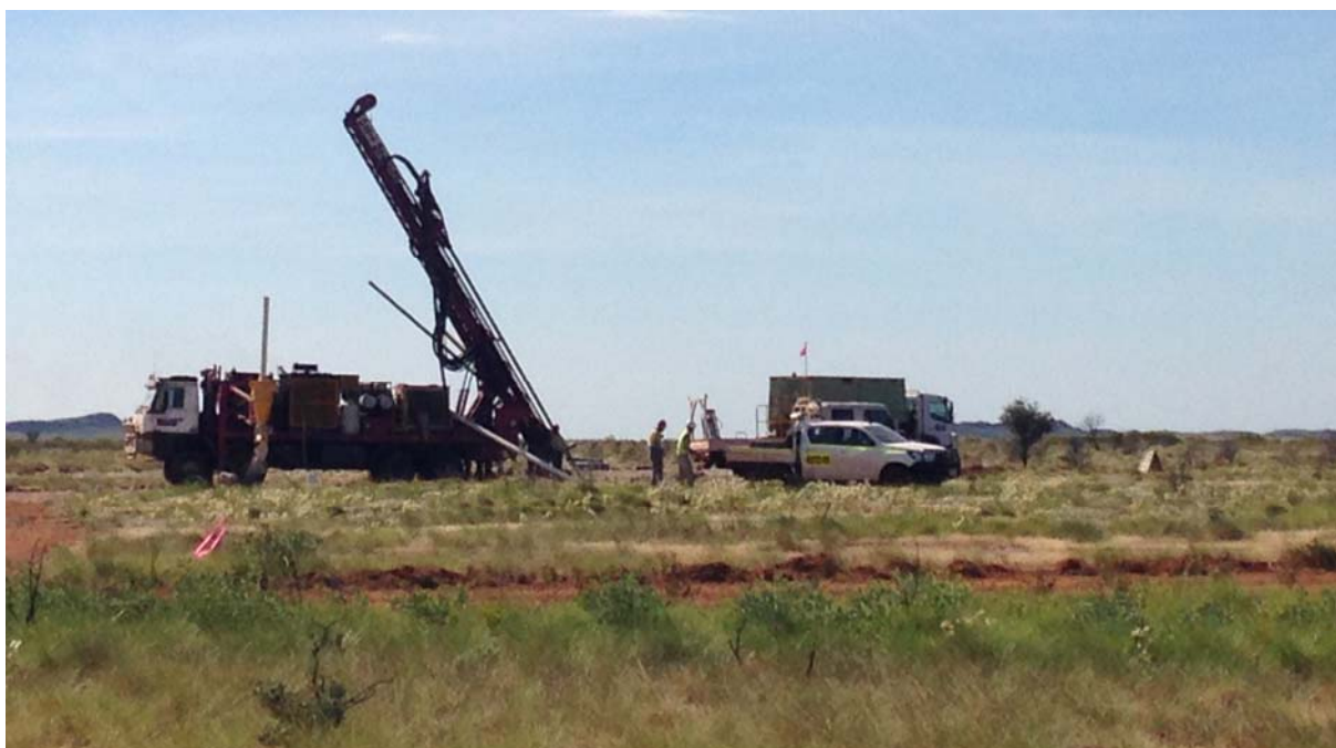
Figure 4 – RC drilling rig on site
