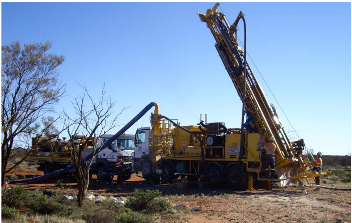
Picture 1.2.1: RC Drilling in the Challenger Matrix
