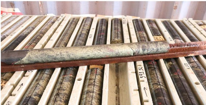
Hole KJCD215 - Zone of semi-massive and breccia of magnetite + chalcopyrite (Conductor 3) circa 592.36 – 593.05 m.
