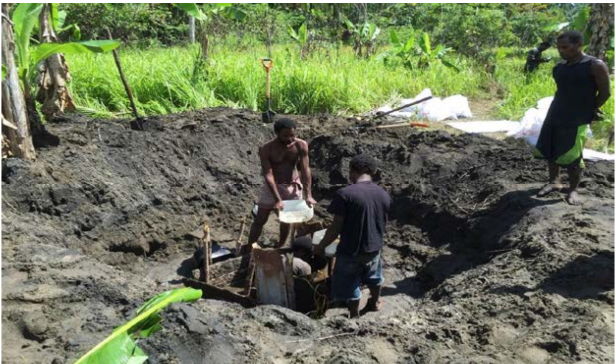
Plate 10: The method of bulk test pitting, which provides for significantly larger samples and geological understanding in contrast to typical small-diameter drill holes.
