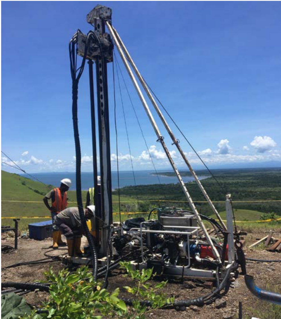
Plate 3: Drilling rig on Kido deposit, where to date up to 100 metres of limestone has been intersected.
