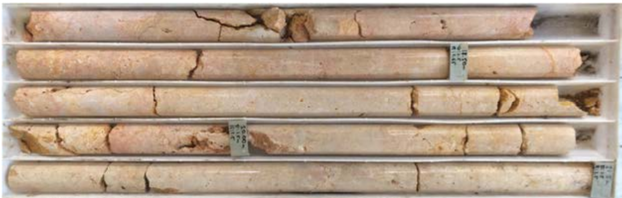
Plate 4: Core hole MRDD005 (Kido) with this material encountered at a vertical depth of 17 to 21.5 metres downhole. The start of the tray is at the top left hand corner.
