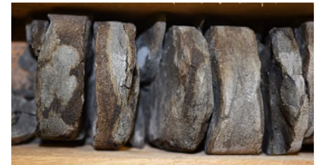
Corehole Achar E-1; Oil leaching from Devonian sandstones just below Cordobes Shales
