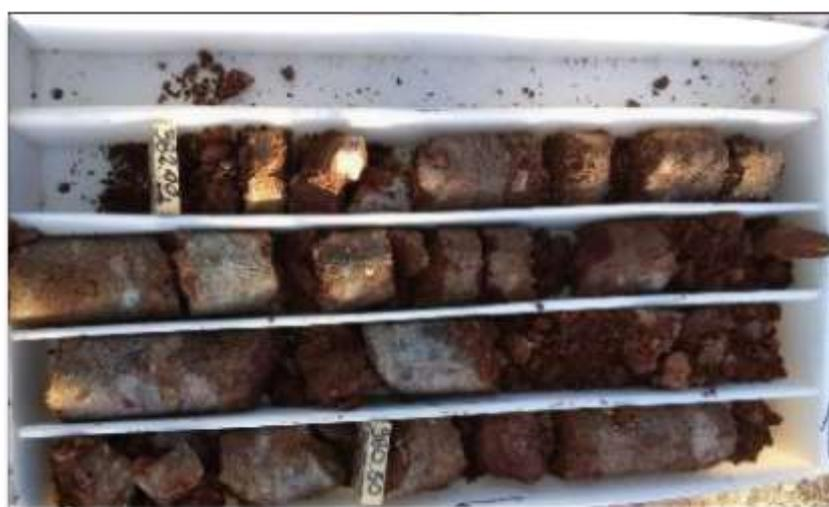
**Figure 3. Recovered conglomerate core from PP2-JV006**
