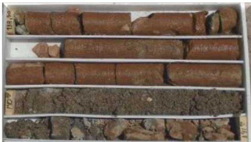
**Figure 2. Recovered unconsolidated core from PP2-JV006 in the south of the project**
