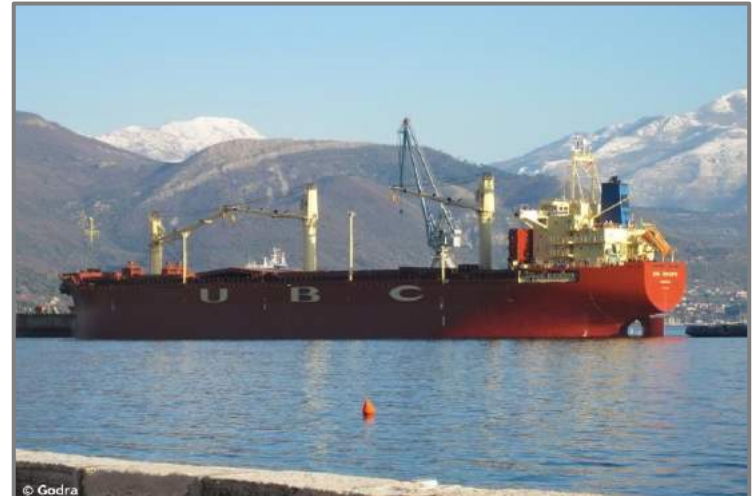
Bulk carrier with pneumatic un/loading
