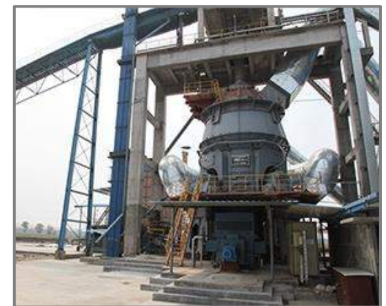
Clinker grinding vertical mill
