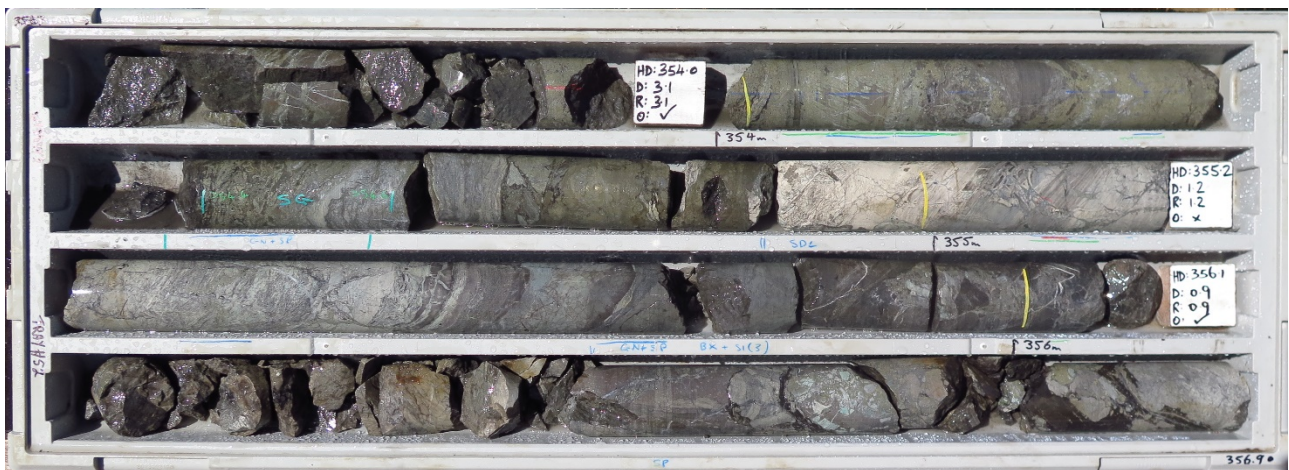
Figure 1. WFPD173 – Re-entered historical hole which was diamond tailed – abundant galena and sphalerite in the upper Py3.
