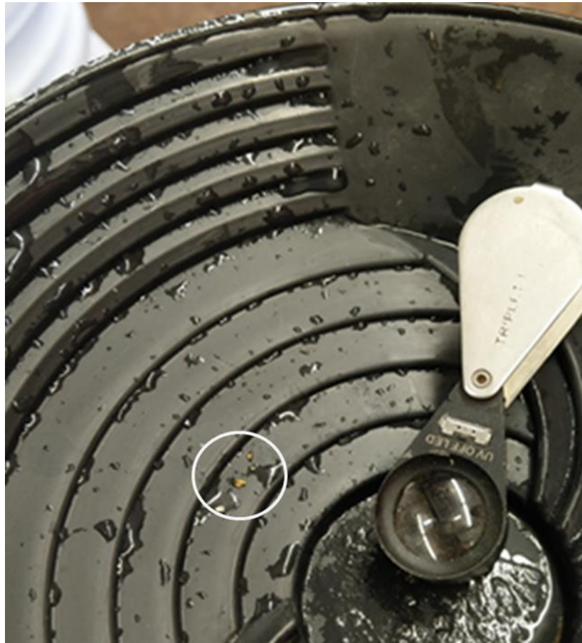
Photo 4. Gold crushed in a traditional dolly pot, from a 10KG sample.
