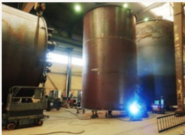
Fabrication commences on the LEILAC furnace sections in Belgium.
