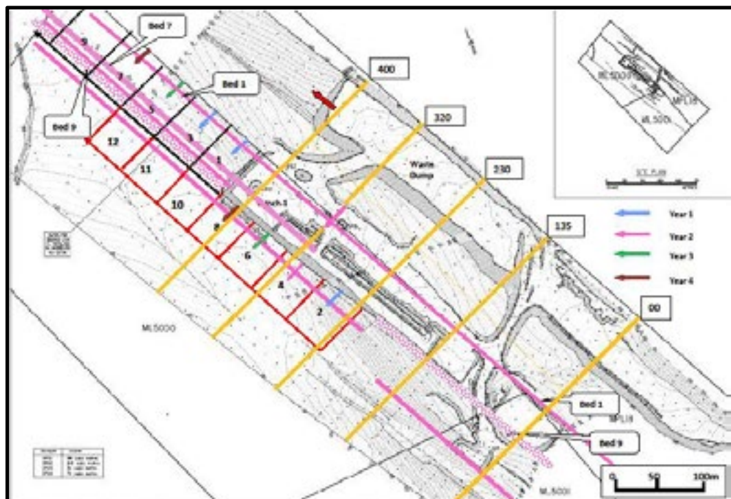
Figure 10: Mining sequence showing panels 1 – 12
