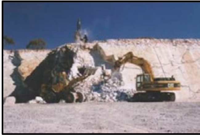
Plate 13: Excavator breaking ore from the face
