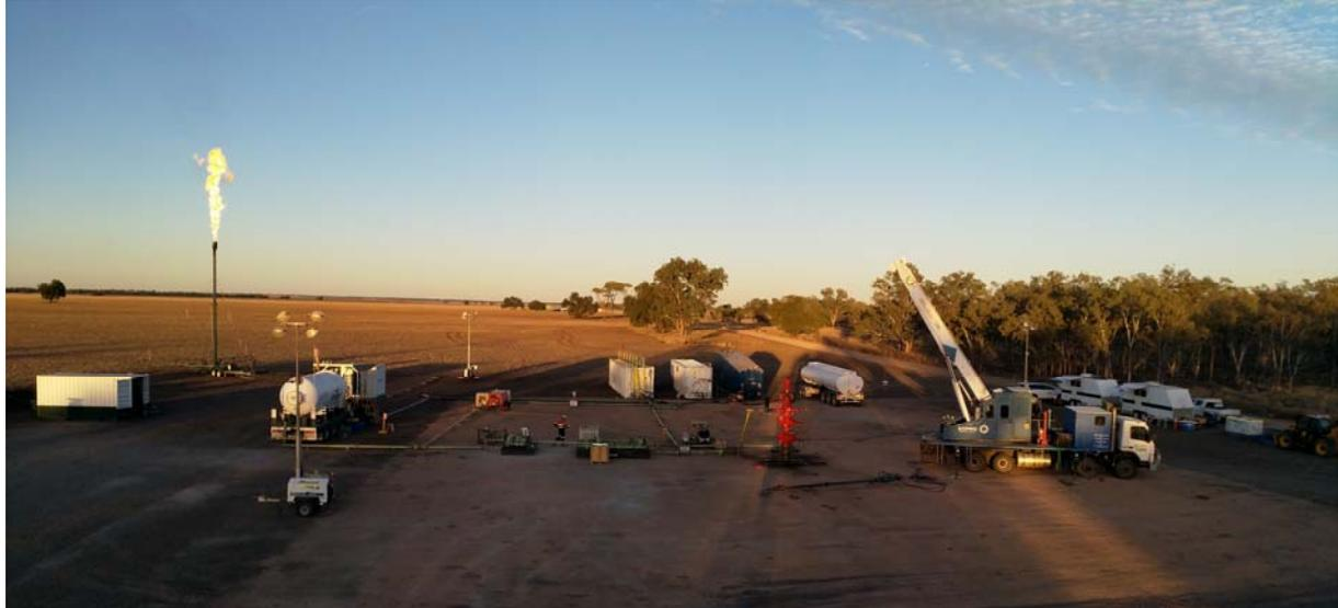
**Myall Creek 4A wellsite – flaring initial gas flows of 2 MMCFD during flow back operations**
