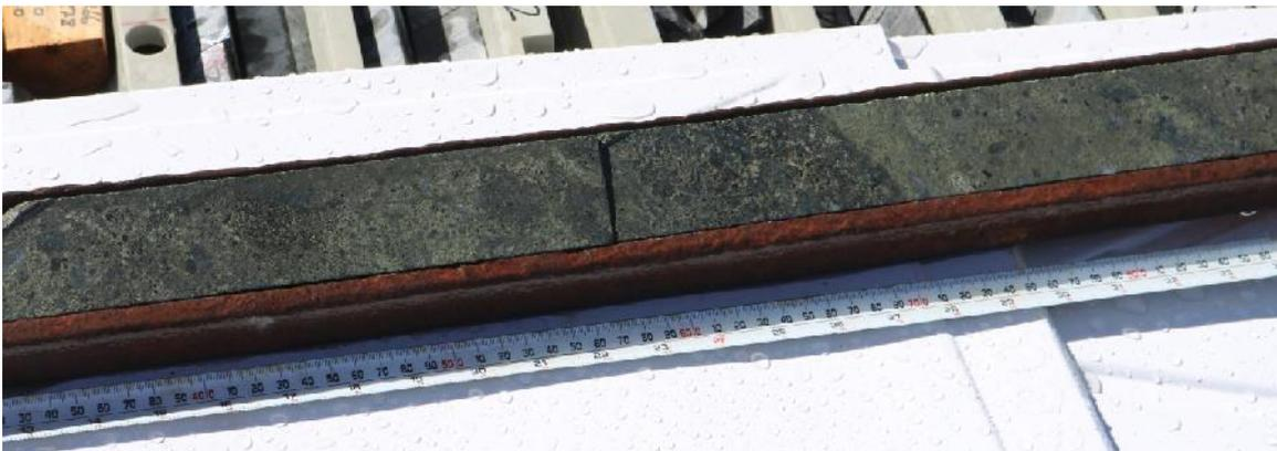
Figure 7 KJCD245D2 – North Lode massive, matrix and disseminated chalcopyrite and pyrite within a zone of magnetite associated with biotite and chlorite. Drill hole depth approximately 438m.
