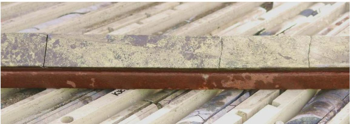
Figure 8 Hole KJCD245D3 – Massive to semi-massive chalcopyrite and pyrite mineralisation with minor carbonate veinlets. Drill hole depth: 705 to 706m.
