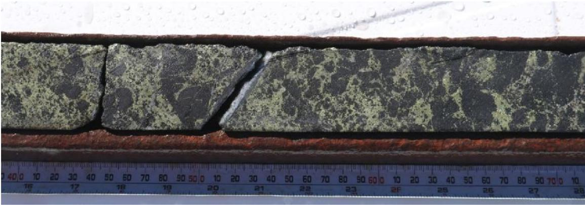
Figure 6 Hole KJCD245D1 – Close up of North Lode mineralisation, with magnetite hosting semi-massive and stringers of chalcopyrite and pyrite. Minor chlorite and biotite alteration is also visible. Drill hole depth is approximately 538m.
