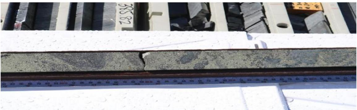
Figure 9 . KJCD245D2 Massive chalcopyrite mineralisation featuring minor pyrite within a psammite. Drill hole depth is approximately 684.6m.
