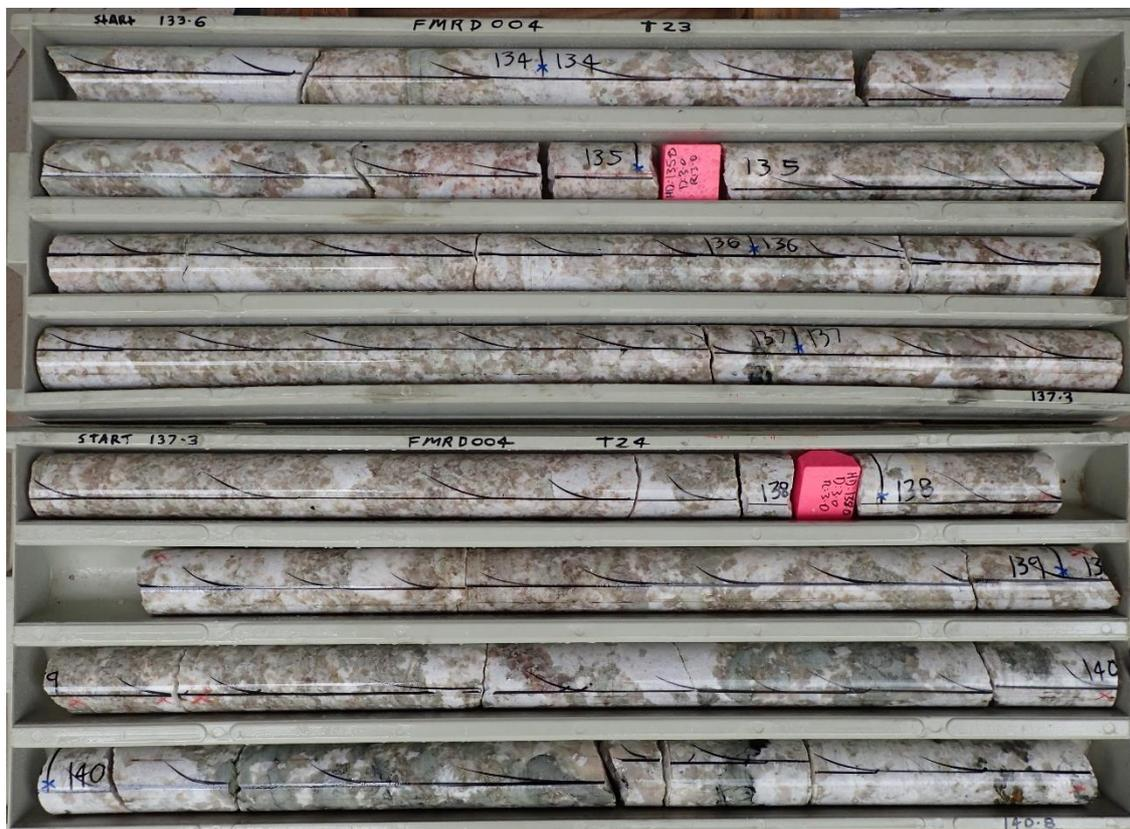
Photo 1. Spodumene pegmatite drill core at BP33 grading at 1.84% Li<sub>2</sub>O from 129m-140m FRMD004.
