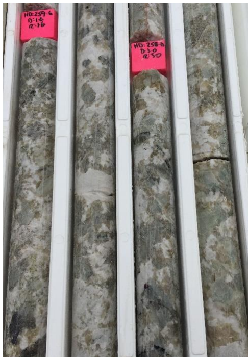
Photo 1 and 2. Coarse green spodumene in pegmatite drill core FRD007, BP33 Prospect.
