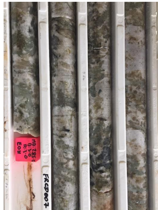
Photo 1 and 2. Coarse green spodumene in pegmatite drill core FRD007, BP33 Prospect.
