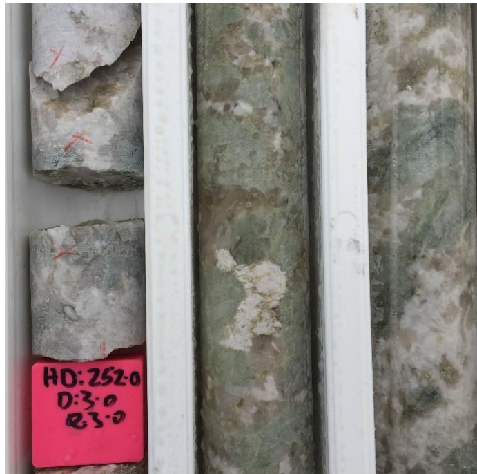
Photo 3. Coarse green spodumene comprising up to 30%-40% of the pegmatite.
