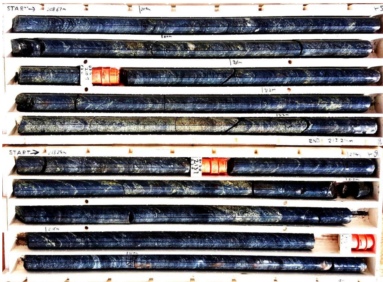
Plate 1 Example of abundant copper mineralisation in magnetite rich rocks in hole 18CB054. Black is predominantly magnetite, biotite and quartz. Yellow-bronze speckle is sulphide dominated by chalcopyrite (copper sulphide).
