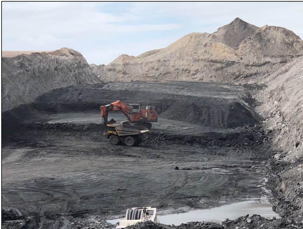
Image: Excavator at Blair Athol loading Run of Mine Coal into haul truck
