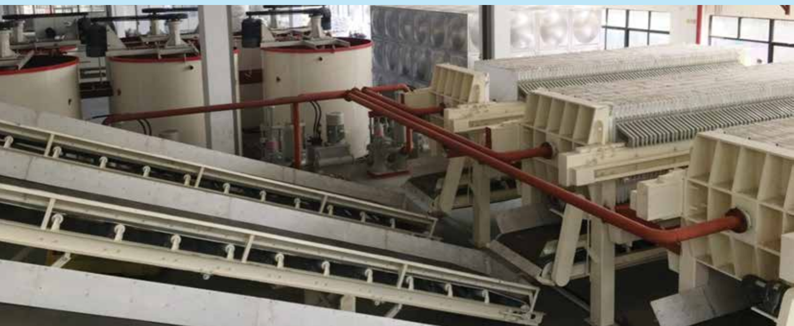
▼ FIRST STAGE OF PRODUCTION – MIXERS AND FILTER PRESSES LEADING BY CONVEYOR TO THE EXTRUDER AND DRYER.
