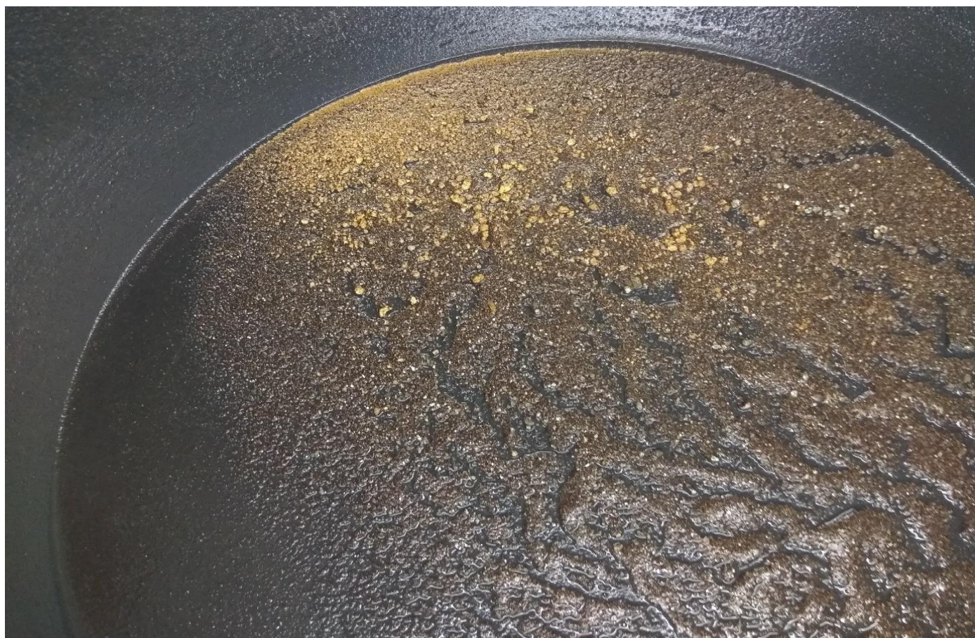
Panned concentrate of drillhole PTAC492 10-12m showing extensive coarse gold recovered. The conventional assay (50 gm fire assay) for this interval was 27.8 g/t Au and the washed gold/panned concentrate result returned 28.22 g/t Au confirming the high gold grade for this interval. Field of view approximately 20 cm.
