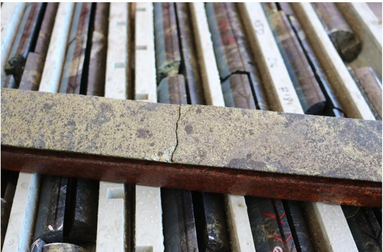
**Photograph 3.** KJCD216 - Massive sulphide zone circa 645.27- 646.67 m.
