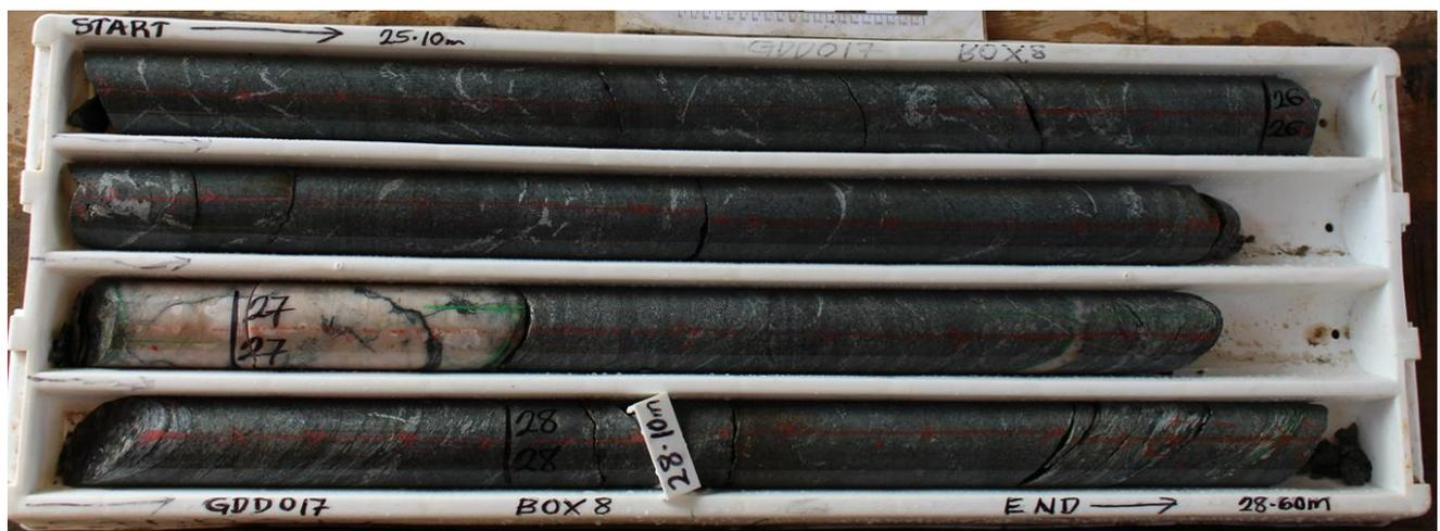
GDD 017 - Quartz veining in a sheared intermediate meta-volcanic @ 25-28m, part of a sequence from 26-29m averaging 2.13 g/t Au.
