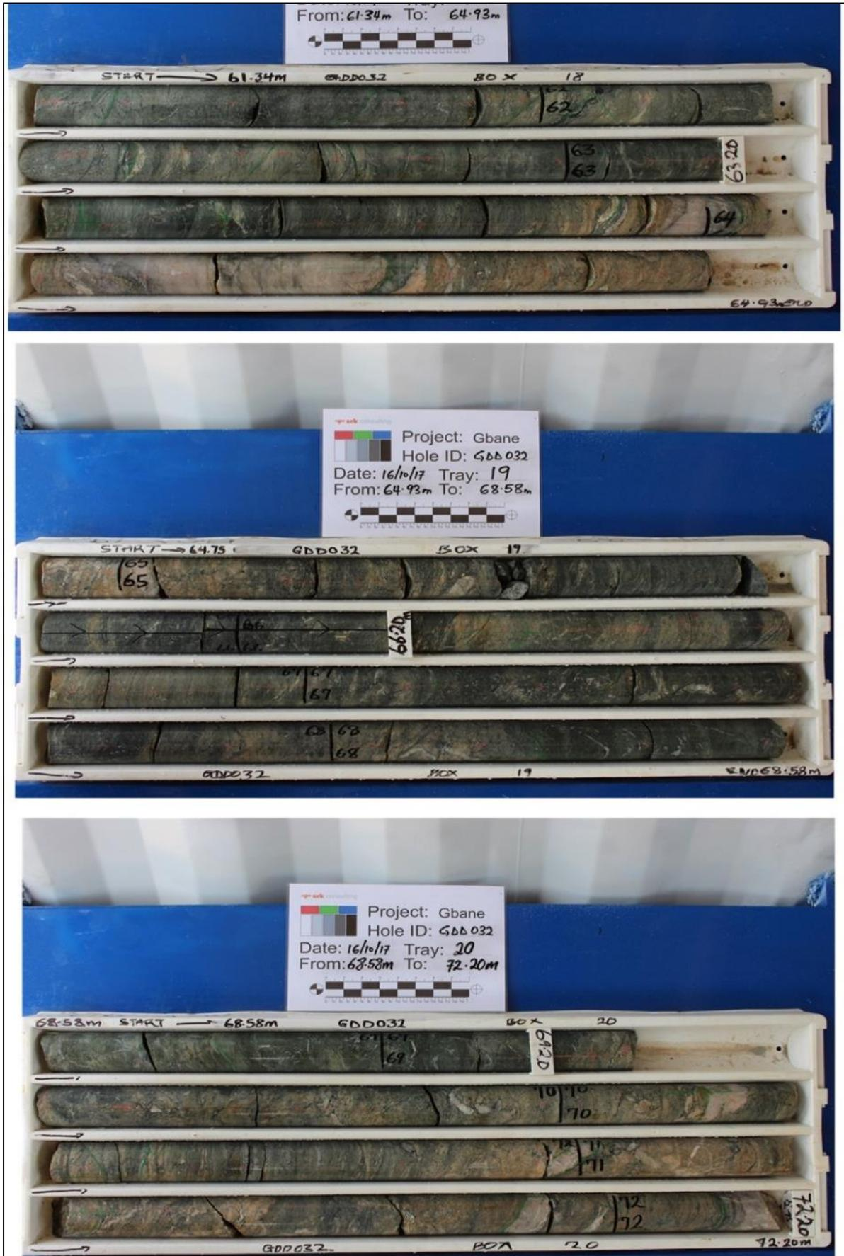
Figure 3: GDD 032 - Intense shearing, alteration and quartz-carbonate veining @ 61-72m, part of a sequence from 63-73m averaging 1.75 g/t Au.
