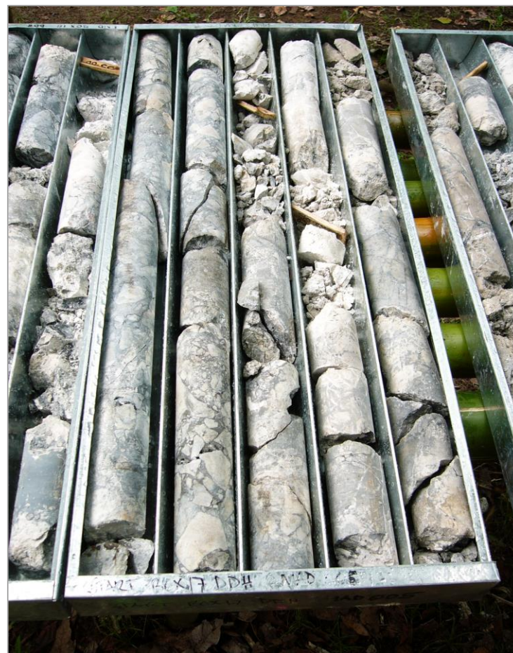
Feni Island photos from Macmin, March 2004. Photo of intensely gold-bearing fluidised hydrothermal breccias. Average grade from 52-60m (depicted within this core tray) was 2.3 g/t Au.
