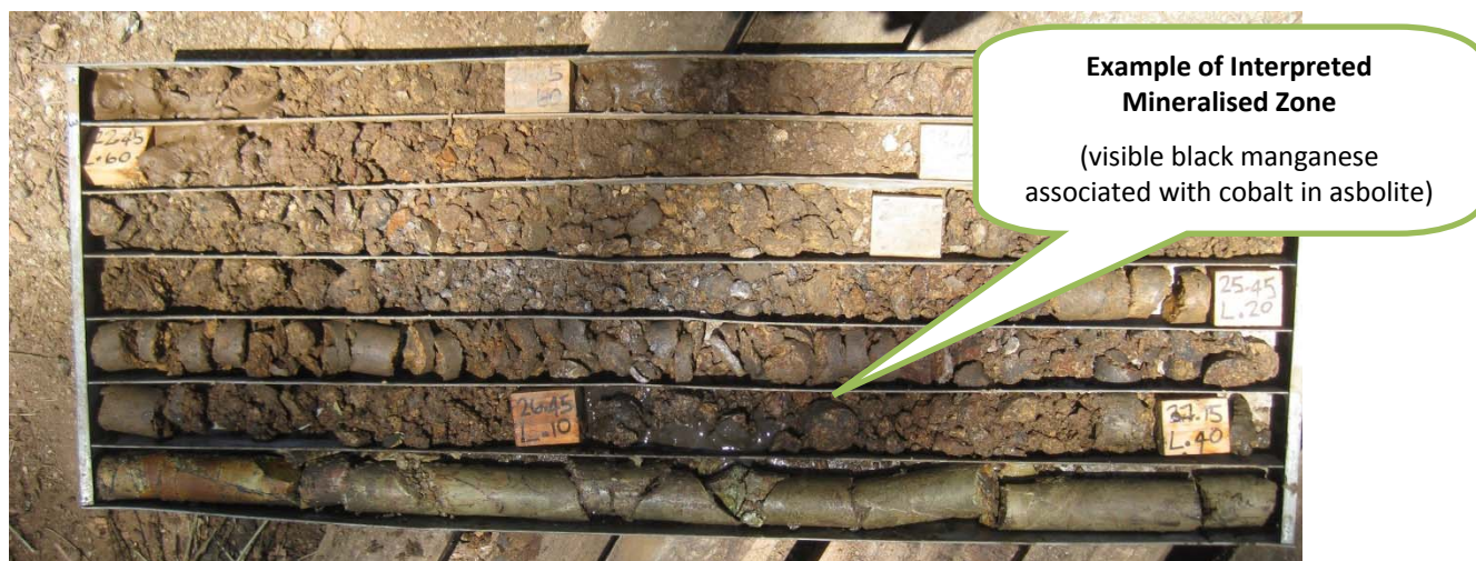
Figure 1 – Section of mineralised zone for COB 029 (22.4m to 27.15m)
