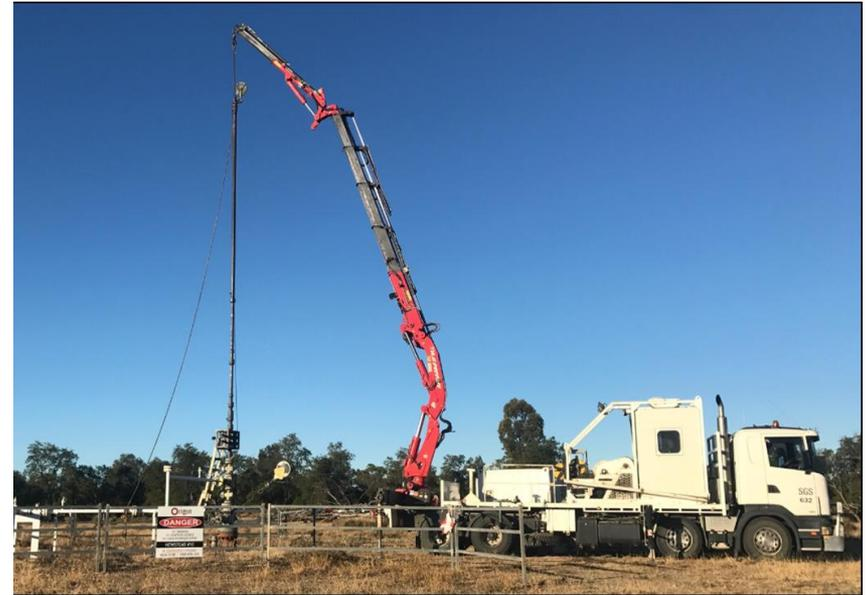
SGS performing static gradient survey on Newstead 10 well, June 2017; confirmed volume (2.3 PJ) and integrity the Newstead storage facility.
