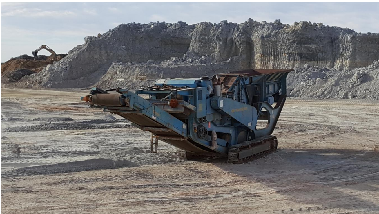
Impactor crusher that will be used to crush the soft high grade ore in the large stockpile in the background.
