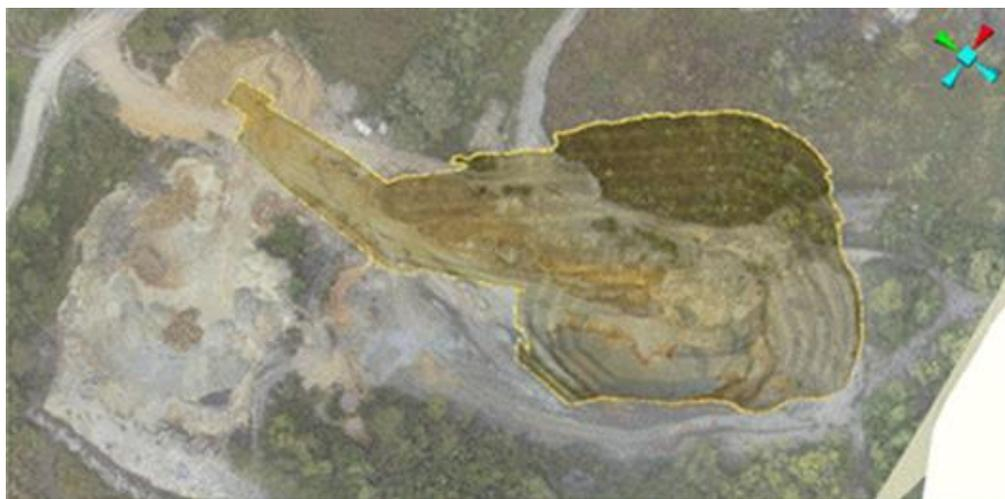
**Figure 2 – Topographical overview of existing Granville East open pit, with proposed east wall cutback superimposed**
