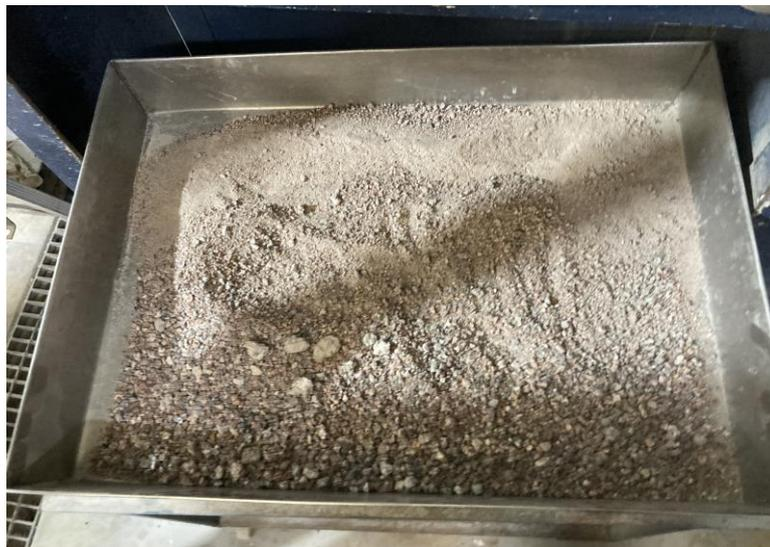
[Figure 1] Example of coarsely crushed core for Phase 2 leach test work.
