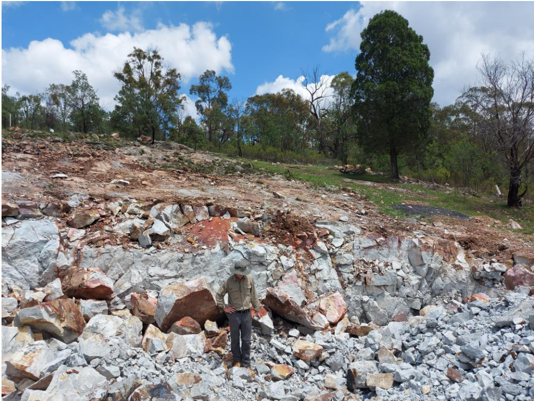
Figure 2: Bulk sample blast site showing mineralised fractures.
