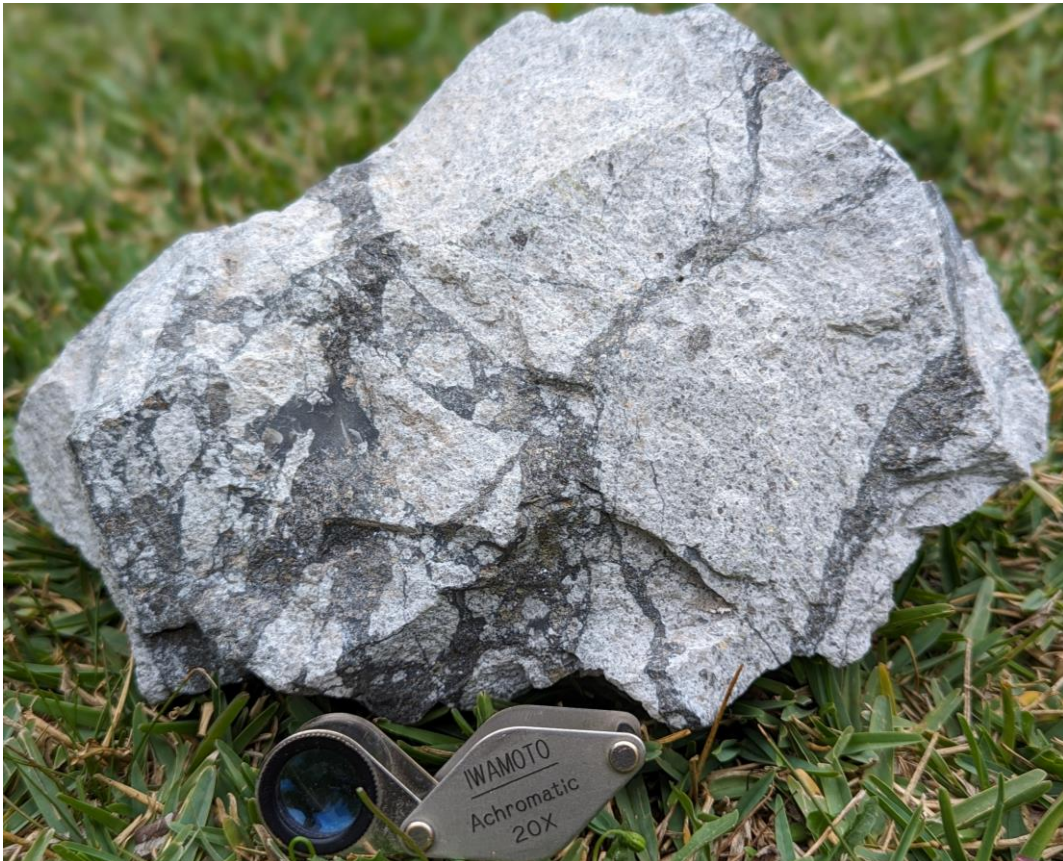
Figure 3: Material from bulk sample site with grey fracture/breccia fill minerals of silver sulphides such as acanthite ( \text{Ag}_2\text{S} ), galena ( \text{PbS} ), sphalerite ( \text{ZnS} ).
