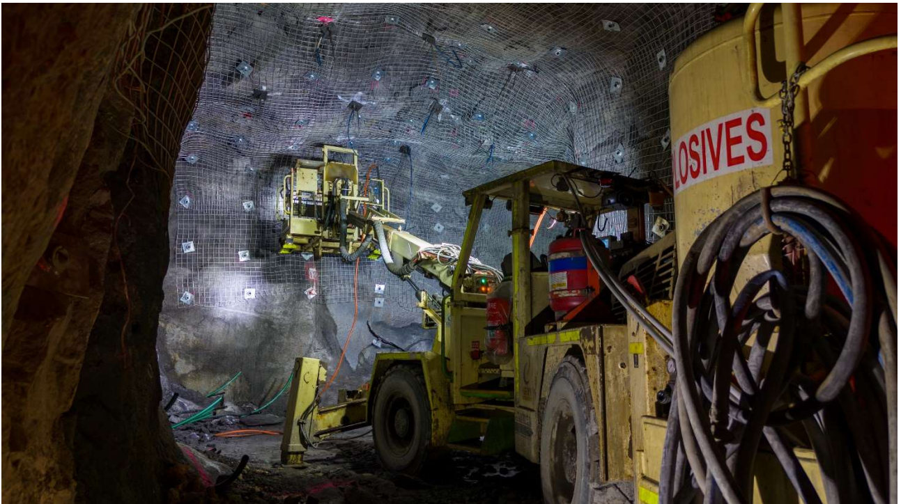
Figure 2 Loading explosives
