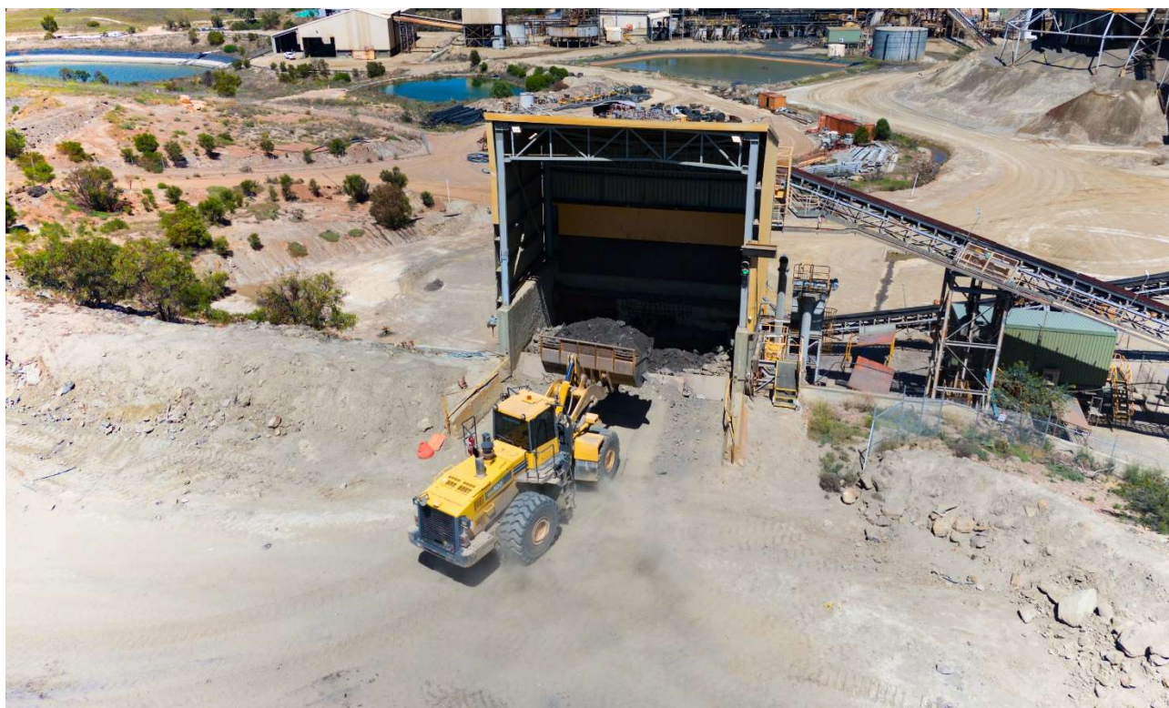
Figure 4 Feeding the crusher
