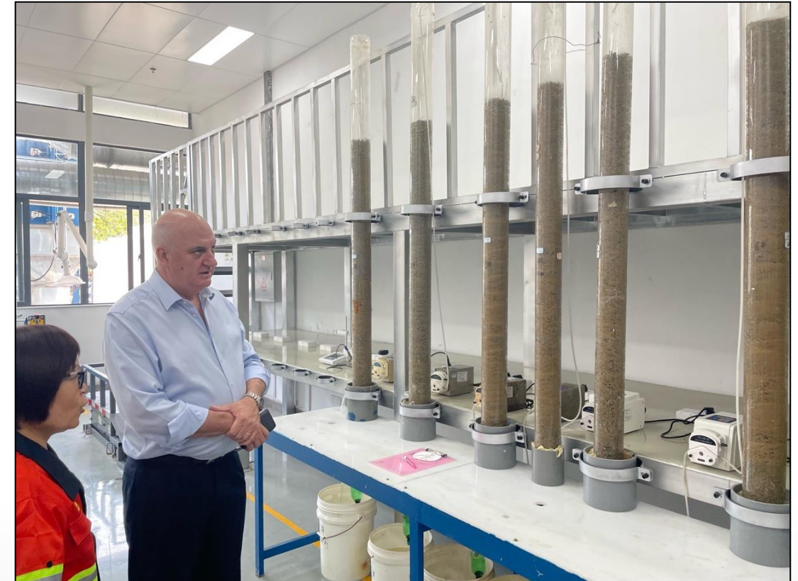
Oxide Column Leach at Zijin Research Labs
