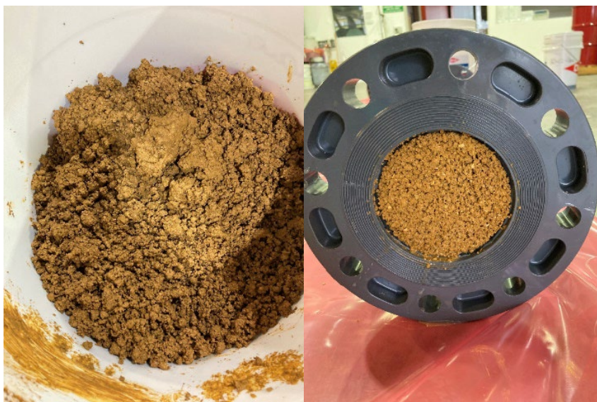
Figure 2: Column 1 clay in bucket post column test & material in column 2 post agglomeration, leaching, wash.
