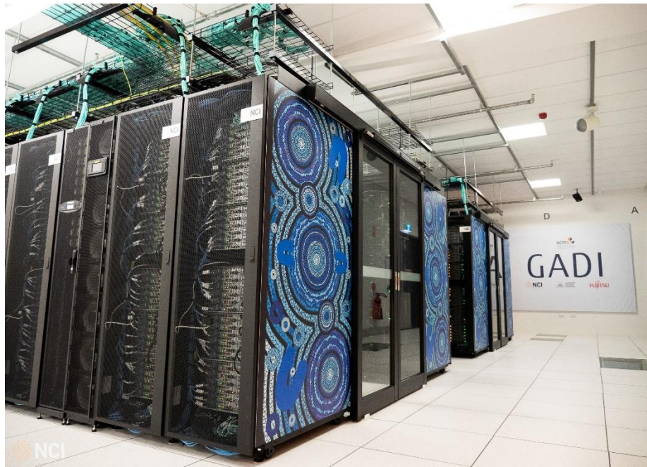
Figure 1: the Gadi supercomputer incorporates rows of CPUs and GPUs within a water-cooled environment to facilitate computing capacity of over 10 quadrillion operations per second.
