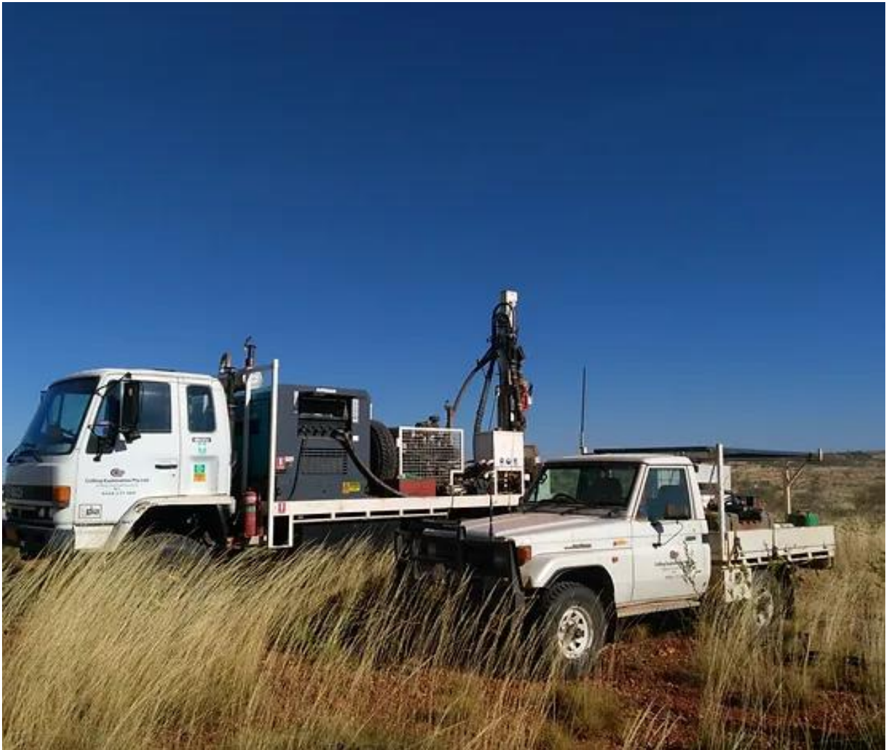
Figure 3: Colling's Drill Rig 2, an Isuzu 4x4 mounted Hydco a30 AC/RAB rig
