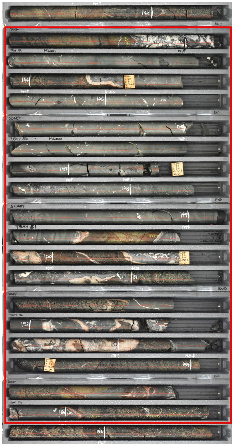
Figure 8: Drill core trays from ML001 showing main zone (red outline) of massive chalcedony vein and breccia with sphalerite-galena+/-chalcopyrite veins and breccia and lesser chalcedony-quartz-adularia veins and vein clasts in sericite-hematite altered porphyritic dacite.
