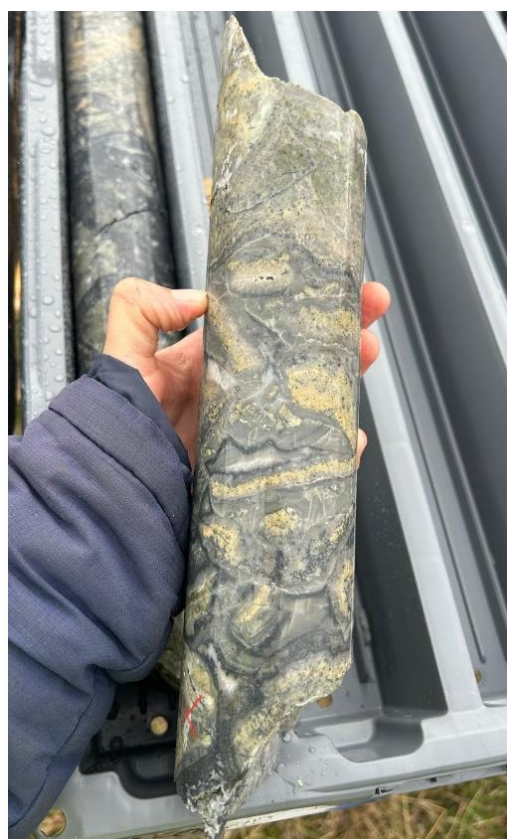
Figure 1 (left): ML001 at 151m - quartz-galena-sphalerite-chalcopyrite-adularia-chalcedony breccia Figure 2 (right): BK002 at 108.6m – chalcedony-quartz-adularia-pyrite-sphalerite-galena cockade breccia
