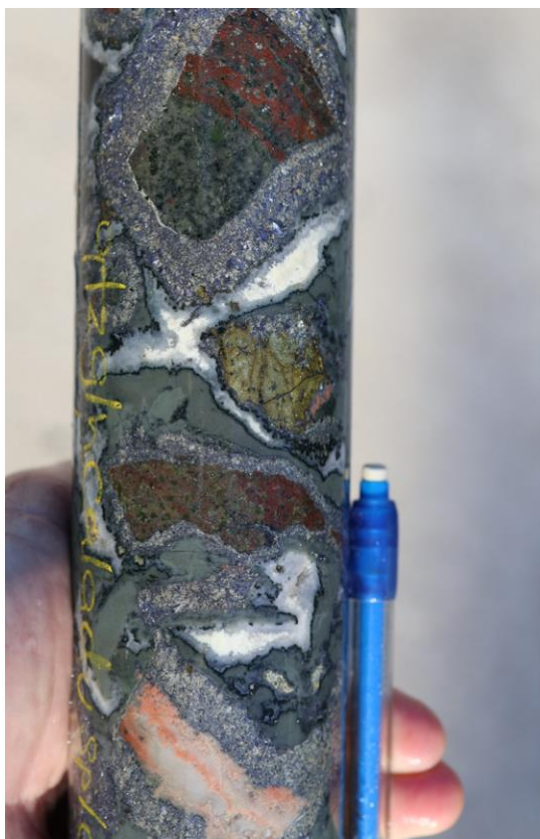
Figure 1 (left): ML001 at 151m - quartz-galena-sphalerite-chalcopyrite-adularia-chalcedony breccia Figure 2 (right): BK002 at 108.6m – chalcedony-quartz-adularia-pyrite-sphalerite-galena cockade breccia
