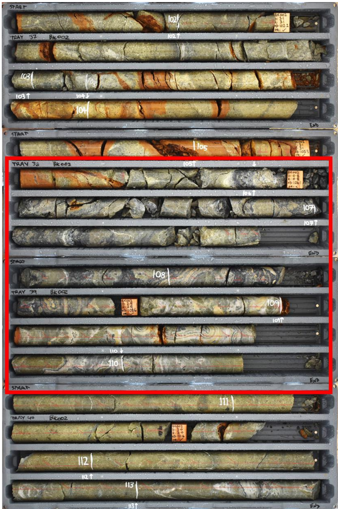
Figure 7: Drill core trays from BK002 showing main zone (red outline) of chalcedony-quartz-adularia veins and cockade breccia which includes fine to very-fine grained sulphide bands as well as sphalerite-galena banding in strongly sericite altered porphyritic dacite.
