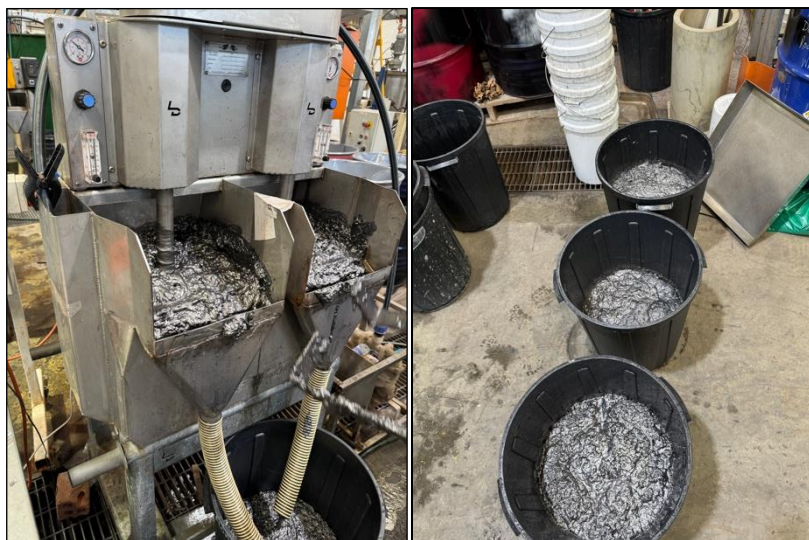
Figure 2. Bulk scale flotation cell (left) with Lacroma graphite flotation concentrate (right)
