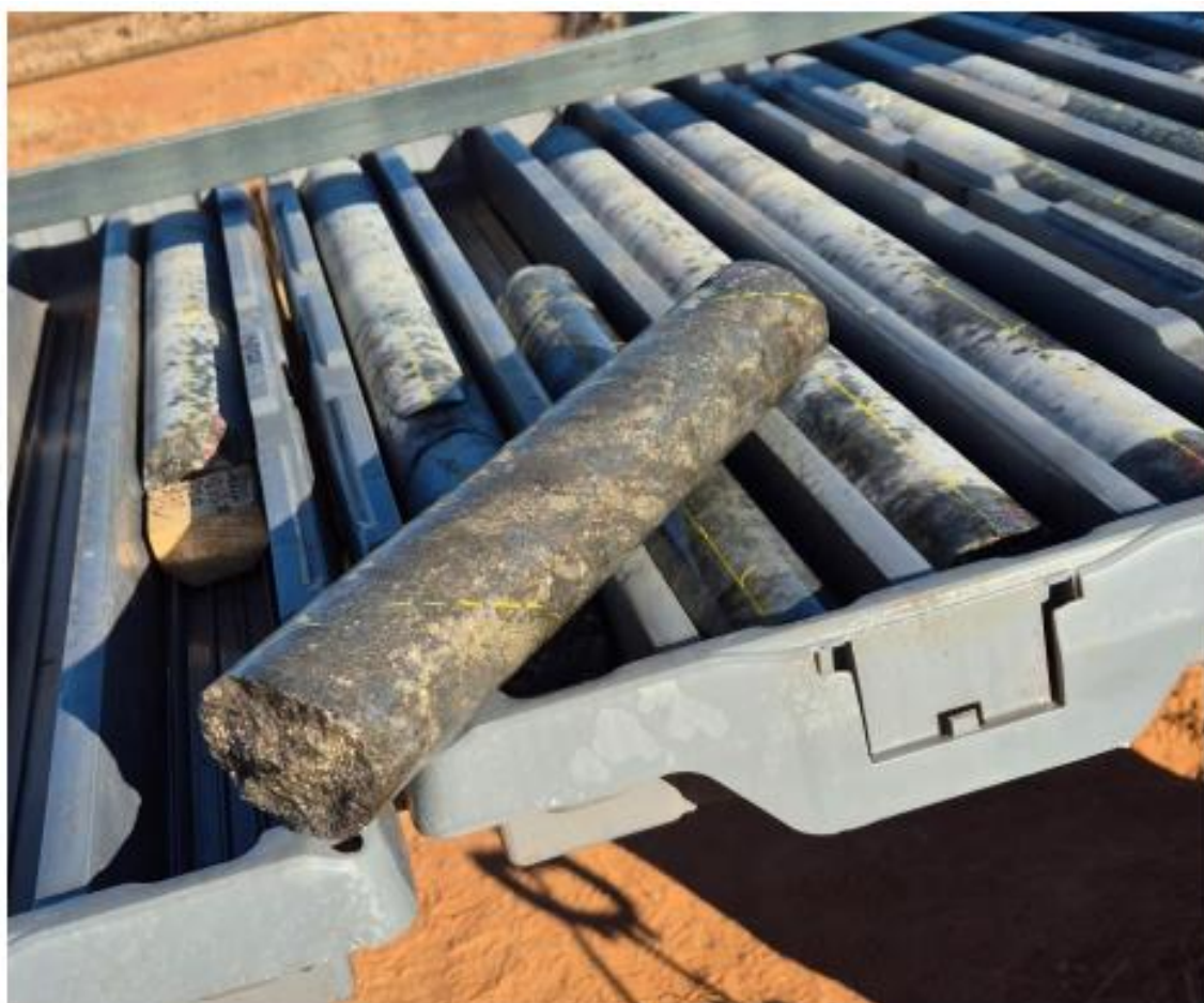
Figure 6 – LMRD002 showing visual semi-massive to massive sulphides from 61.2m to 62.m assay.
