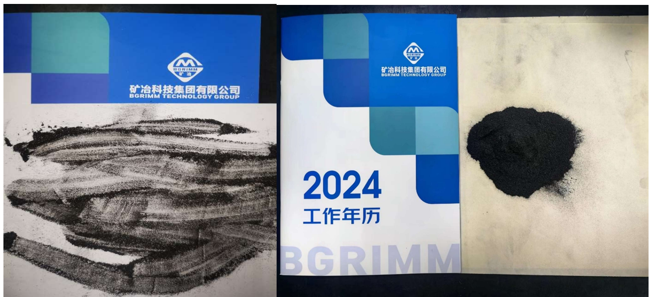
Figure 1. Graphite concentrate produced from the metallurgical samples from the Oar Graphite Project.
