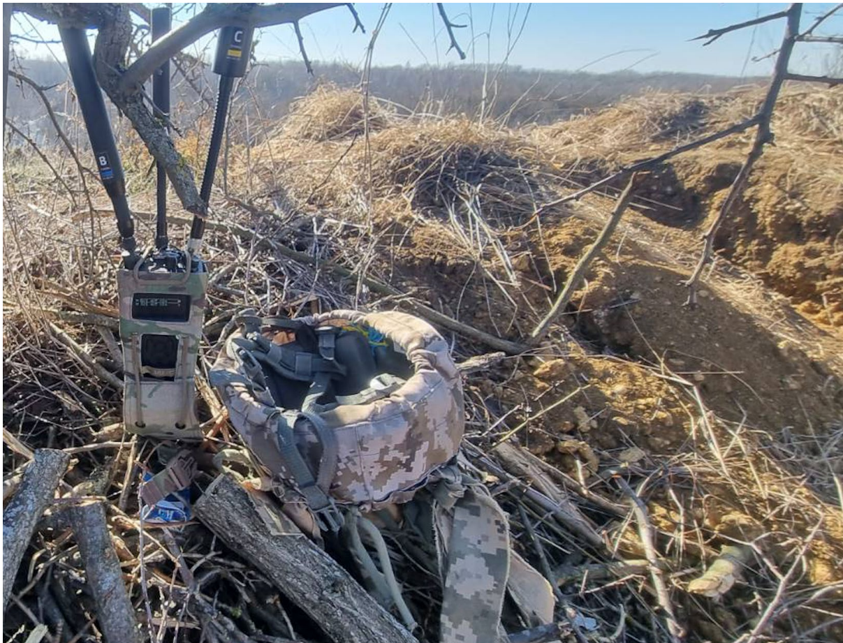
Image: RfPatrol handheld drone detector deployed by a Ukrainian soldier
