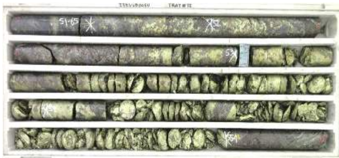
Figure 7 Cu-Au mineralisation in 23KVUG064 through the East Kavanagh Lode
