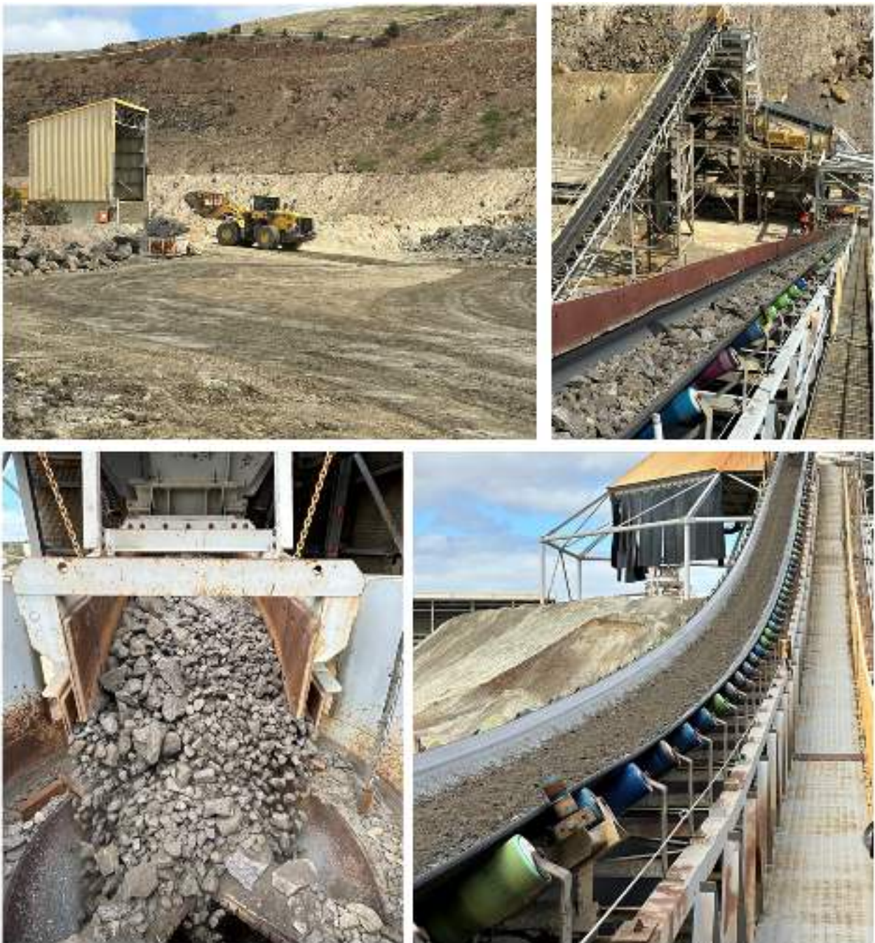
Figure 6 First crushing campaign as part of dry circuit commissioning
