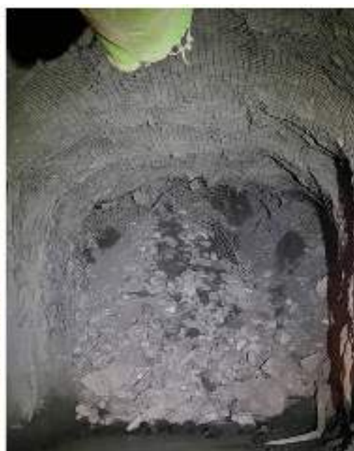
Figure 4 Drilling the first stope (LHS) and drawpoint after firing
