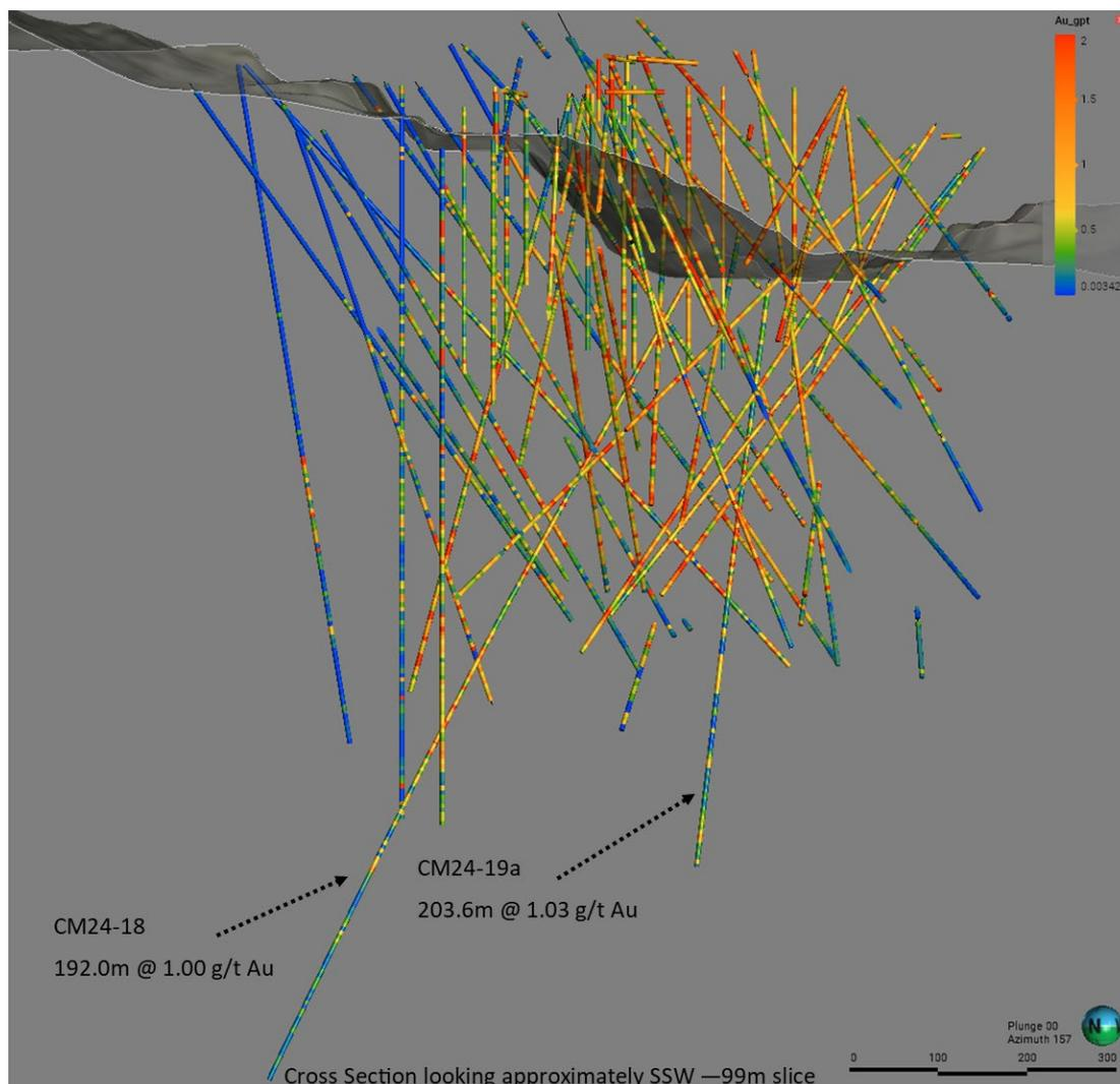
Figure 2: Cross section looking SSW through the north Pipe at Colosseum
