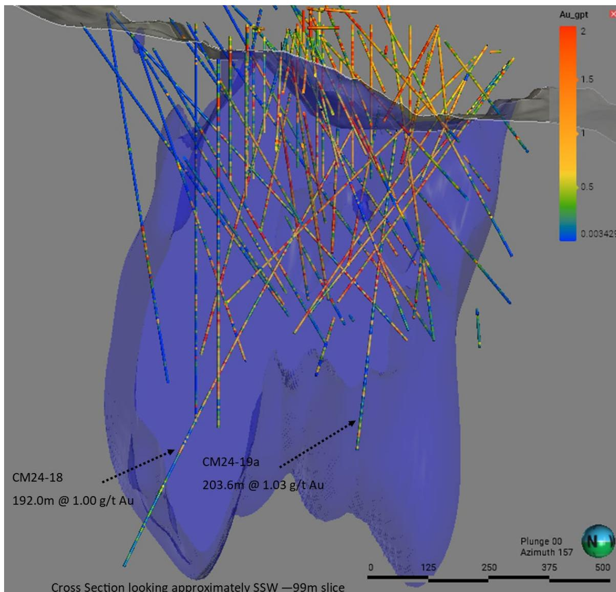
Figure 3: Cross section looking SSW showing the outline of the breccia pipe in blue
