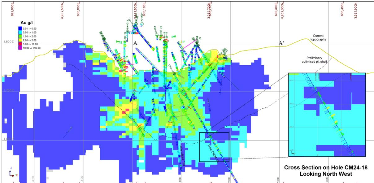
Figure 4: Section A-A' showing drilling grades vs block model grades
