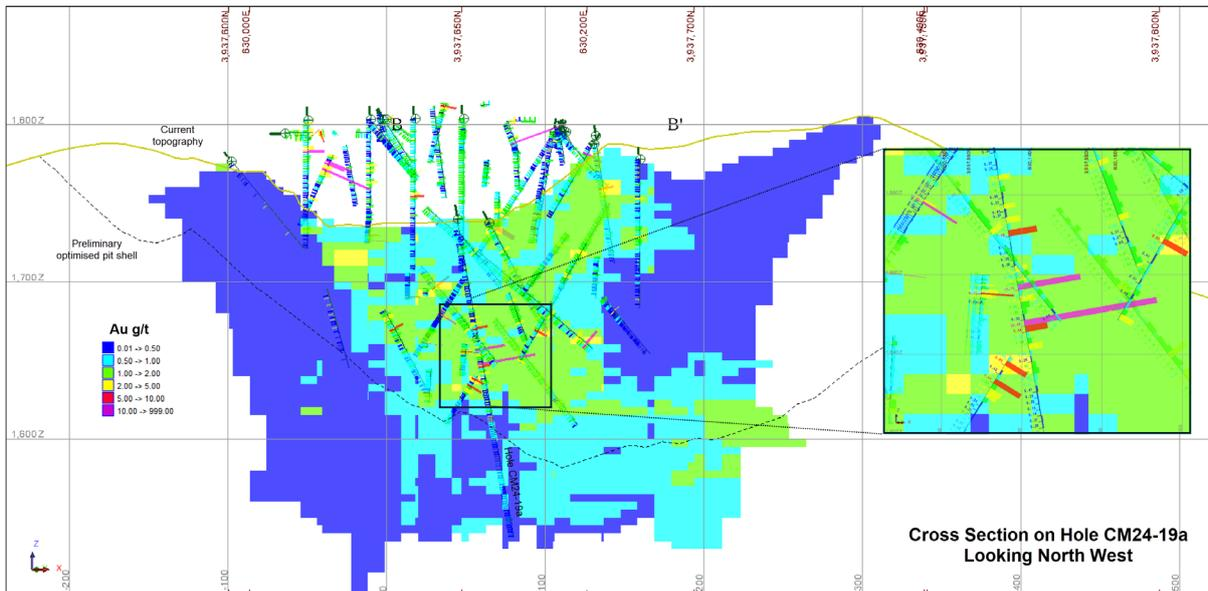
Figure 5: Section B-B' showing drilling grades vs block model grades
