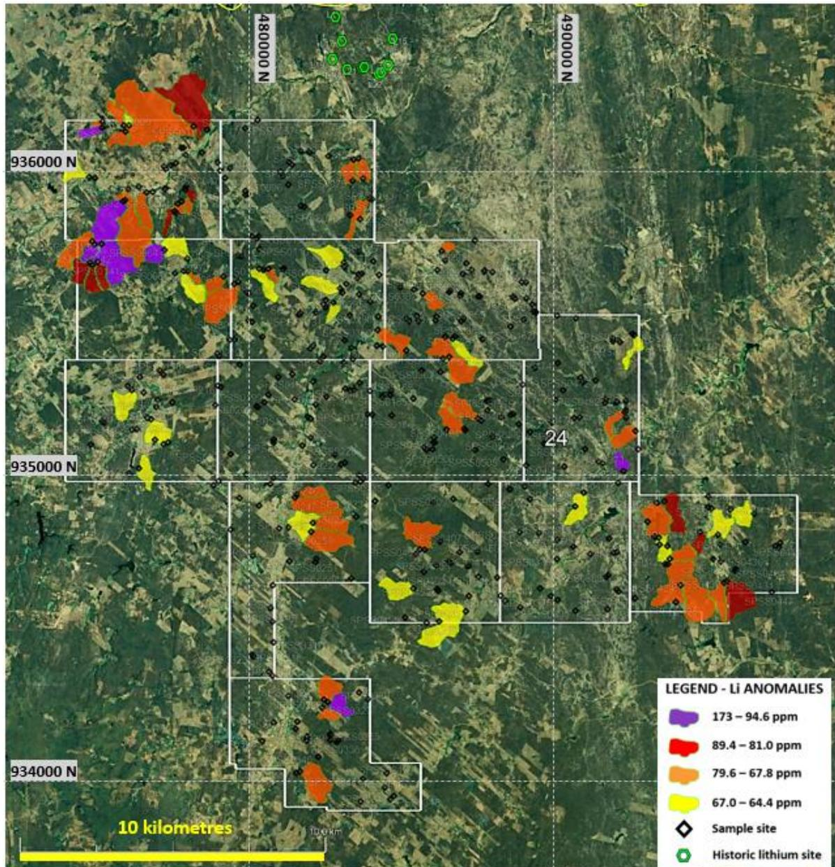
Figure 2. Lithium anomalies plotted as anomalous stream sediment catchments. Maximum value of 173 ppm lithium. Sites with lithium mineralisation potential are shown clustered in several areas, with pathfinder element patterns suggesting series of subparallel northerly trending zones, similar in orientation to the historical lithium occurrences.
