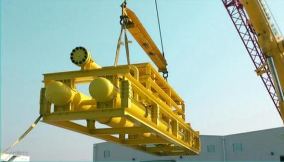
PDG is a series of subsea, inline, piggable devices that enable the economic development of gas discoveries at step-out distances of up to 300km, almost double what can be achieved with conventional approaches
