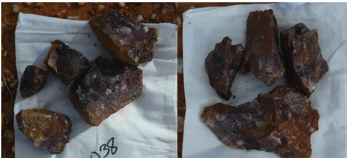
Figure 7. Examples of rock chips taken for gold mineralisation at the Falchion Gold Prospect.
